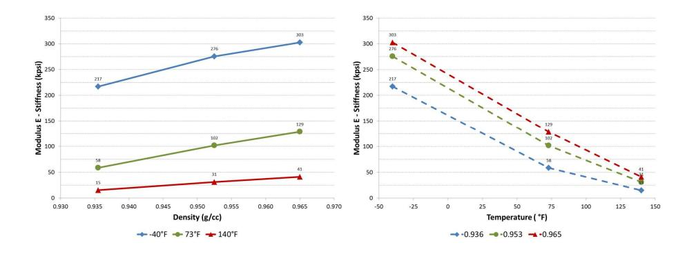
Effect of temperature on stiffness is significantly greater than that of resin density
