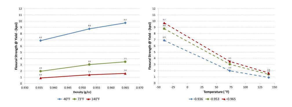
Effect of temperature on flexural strength at yield is significantly greater than that of resin density
