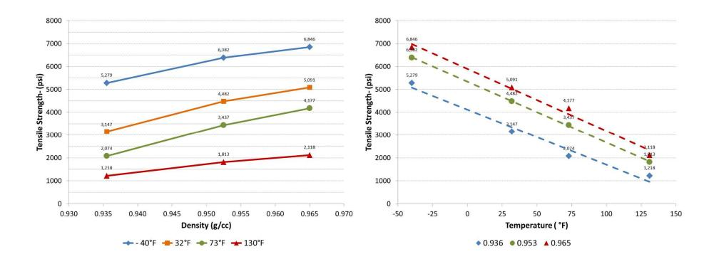
Effect of temperature on tensile strength is significantly greater than that of resin density
